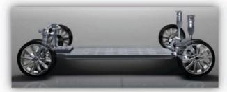
Simple elegance is under the body of Tesla's Model S. The batteries are under the floor for low center of gravity and terrific handling.
